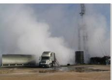
The subject well was undergoing some diagnostic activities, to attempt to locate a suspected hole in the production casing string. There was a workover rig on the hole, with a tapered tubing string and packer assembly. The rig crew was in the process of tripping out of the hole when the well began flowing. The pipe rams were closed and did not stop the flow. The rig was evacuated and Cudd Well Control was contacted to assist in regaining control of the well.
